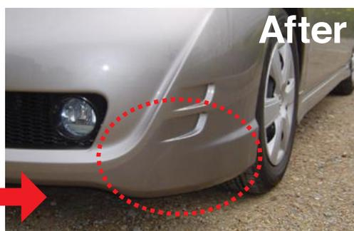
● Mold from the back of the bumper with Sun Sheet.
