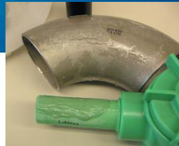
Uni Solar Hard for repair of pressure part such as pipings.
