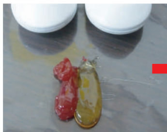
Take the same amount of base resin and hardener.
